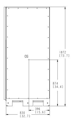
Figure 3-9. UPM Section Center of Gravity
